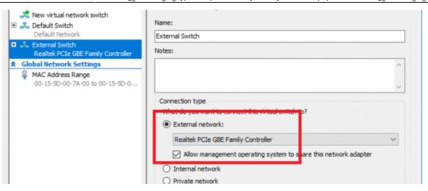
Connect the external switch to the converted virtual machine:
