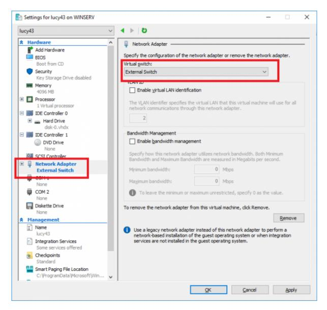
Power on the virtual machine and reconfigure the network:
