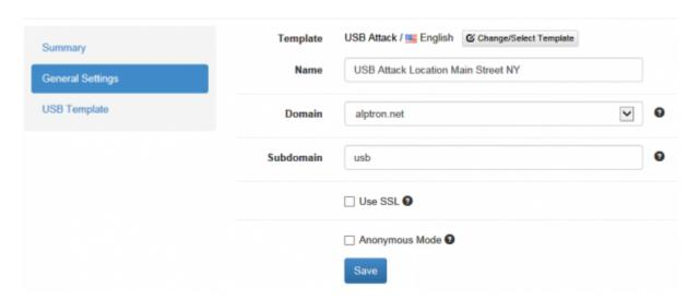
• Next configure the USB template. This template defines what malware simulation should be running upon execution of the file on the USB drive. Make sure you have the latest malware simulations installed in LUCY. You can download the malware simulations using the "download" button in the template section.
