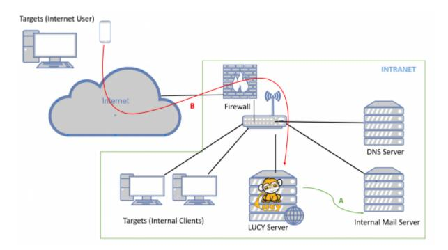
A secure design requires that the web service which is accessible from the internet (untrusted network) can be segregated from the internal network (trusted network) and moved to a DMZ. If you do so, please keep in mind that LUCY has different communication channels that depend on the specific use:
